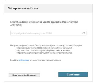
Enter the address at which you will access the BIM Server. This will be the "Primary Address" shown in BIM Server Manager.
