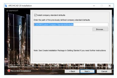
Check **Install Company Standard Defaults**, and enter the file path location of the Defaults folder (containing Work Environment/Translators/Templates) which you created earlier. (See <u>Create "Defaults" Folder</u> at Step 7 above.)
